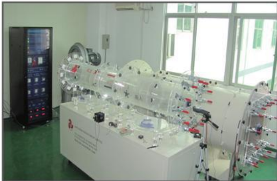
风动测试仪 (CFM test system) Can get the CFM data, mmH 2 O data, working Curve autoly.
